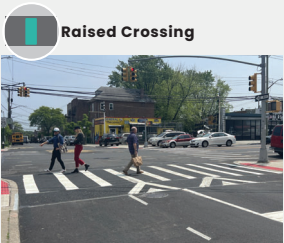
An elevated pedestrian or bike crossing designed to slow vehicles.
