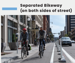
A dedicated space for biking typically separated with a vertical barrier.
