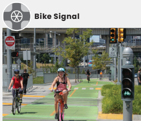
Dedicated traffic lights for cyclists that protect bicyclists from right-turning vehicles.
