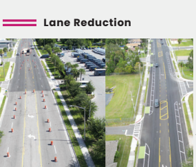
Repurposes a vehicle lane for other uses like bike lanes or wider sidewalks.
