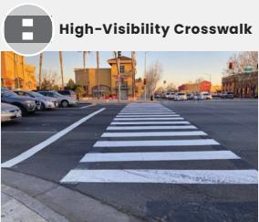
Bold pavement markings to indicate where pedestrians can cross safely.
