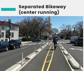
A dedicated center running space for biking typically separated with a vertical barrier.
