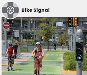
Dedicated traffic lights that help protect bicyclists from right-turning vehicles.
